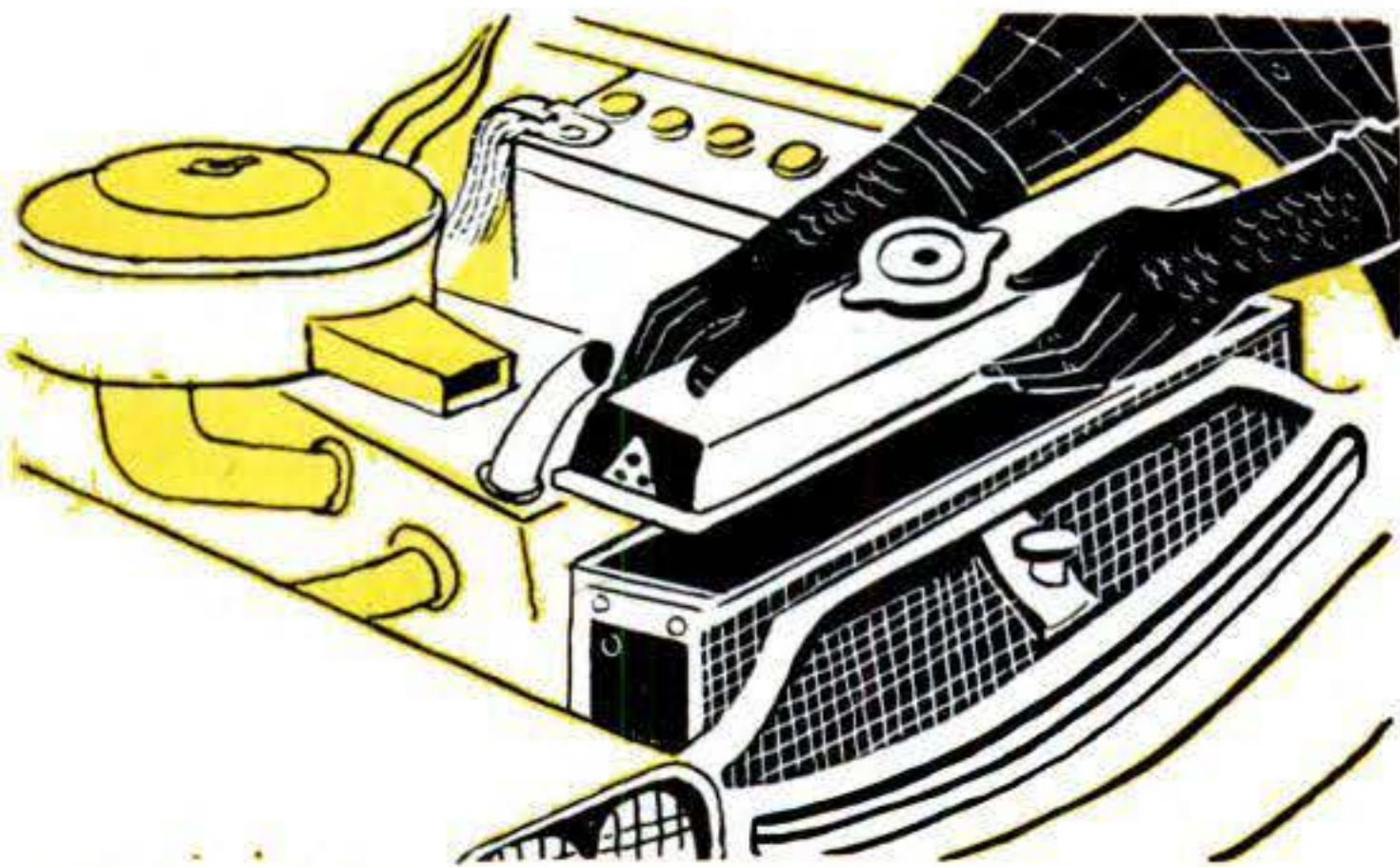
COME-APART CAR RADIATORS with a top chamber that comes off like the oil pan of the engine. Then you could do a complete radiator-cleaning job at home.— L. J. Bump, Vineland, N.J.
